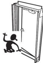
8. Attach threshold anchors
