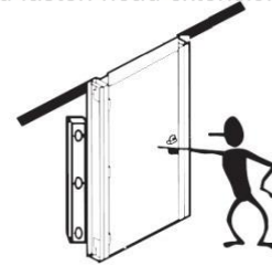
3. Plumb & square door and fasten head extension
